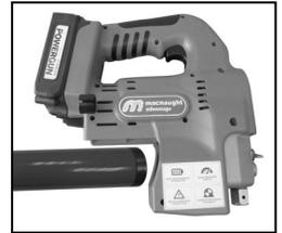
**Note:** Rotate the barrel counter clockwise to remove. Turn clockwise to tighten.
