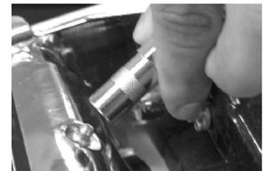
6) Press the trigger on the gun to dispense grease as required.
