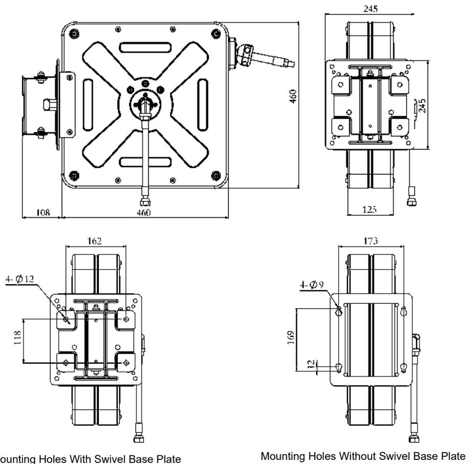
Mounting Holes With Swivel Base Plate
