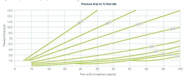
Note: For viscosities greater than 1000 cPs High Viscosity rotors are required
