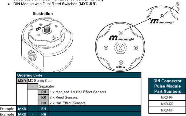
The DIN Compact Pulse Modules accommodates the choice of either a field mountable connector facility, or a fixed (M12) connection cable.
