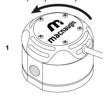
Place pulse cap onto the body and rotate 90° clockwise to reassemble
