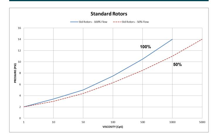
Figure 7: Impact of viscosity on pressure loss for a range of flow rates
