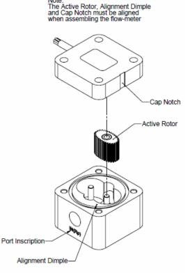
Note: 'CR' Range has a notch in the body not an alignment dimple.
